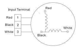
2.Outdoor DC Fan Motor(control chip is in fan motor)(For MSR1U-09HRDN1-QRC4W and MSR1-24HRDN1-QRC4W)
