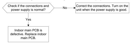
9.2.4 Fan speed has been out of control diagnosis and solution(E3/F5)
