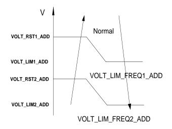
The PCB will detect the voltage of power supply and adjust the compressor running frequency to protect the system.
