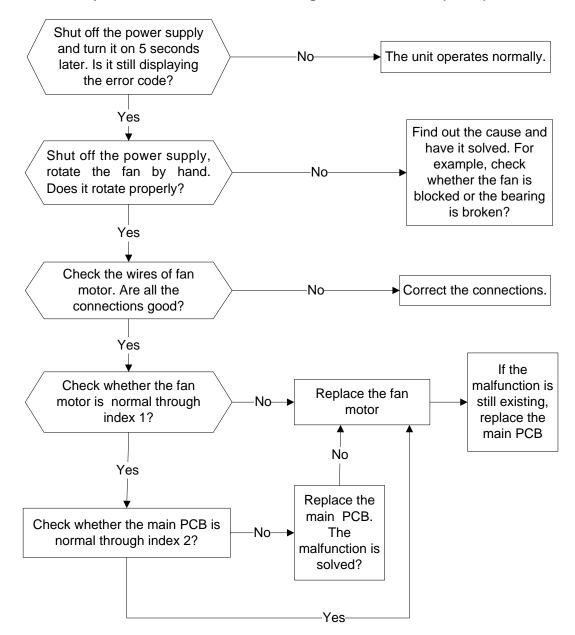
Index 1: 1.Indoor AC Fan Motor Measure the resistance value of each winding by using the tester.
