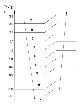
While the zones of A,B,C... are corresponding to different compressor running frequency.
